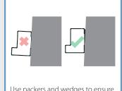
Use packers and wedges to ensure the frame is level and square.
