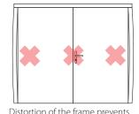
Distortion of the frame prevents good sealing, latching and locking.
