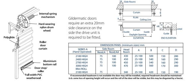
**Sizes** - Up to 5 metres wide and 3 metres high (up to 4.9 metres for B-series – ask for details). Requires no frame so enables the maximum possible opening width for the wider vehicle. Door sits behind the brickwork so can be fitted in arched and unusual garage door openings.
