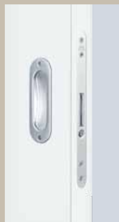
For sliding doors that run within the wall, you can conceal the door leaf completely in the wall with a trip handle. The handle springs out at the press of a button, allowing you to close the door.
